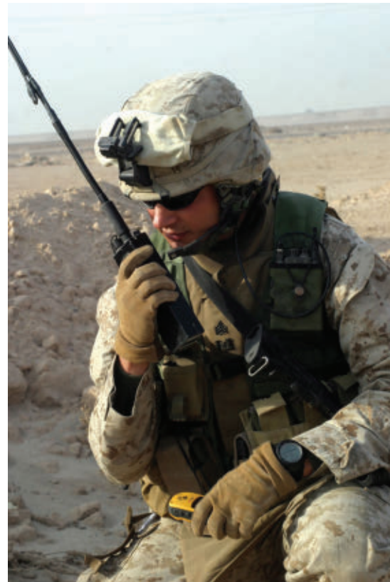
The Air Force is considering developing a Link 16 handheld radio no larger than the AN/PRC-148 multiband inter/intra team radio (MBITR), shown above.
