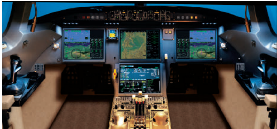
The popular Dassault Falcon sports Honeywell’s EASy II flight deck as its man-machine interface.
