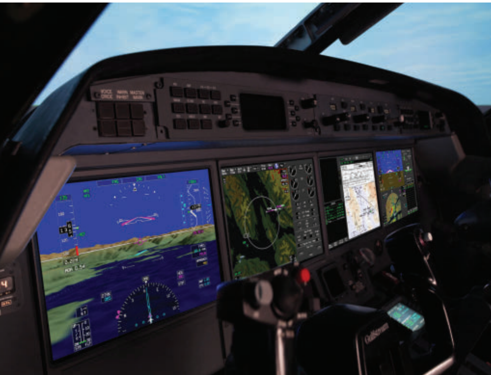
Myriad civil and military aircraft take advantage of modern avionics from technology providers such as Honeywell. Honeywell's synthetic vision system is shown above in a Gulfstream cockpit.
